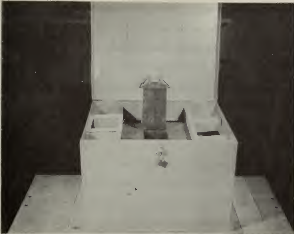
Figure 10 - Source transportation dolly. Shielded volume, 2" deep by 4" square. Shield, 8" thickness lead all directions. Total weight, 2000 lbs.
